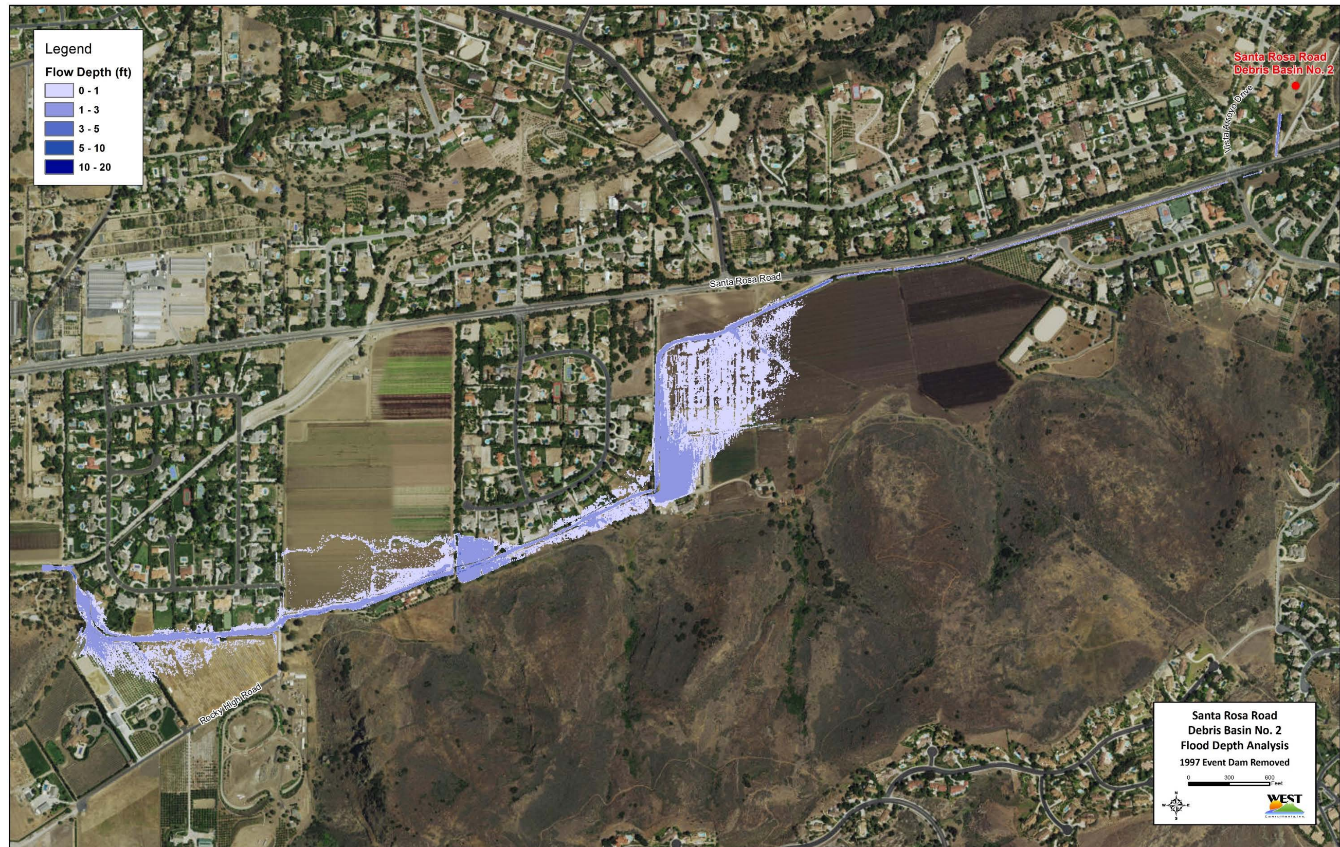
Figure D-2. 1997 Event Inundation Extent, Dam Removed.
